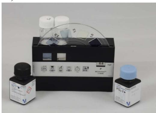
**Hints:** The intensity of the blue complex depends on the concentration of phosphate in the solution. The more phosphate is present, the darker the blue color is. Optionally, one has to dilute the solution and test again. The MColortest is working in the concentration range between 0.2 – 3.0 mg/L phosphate.
